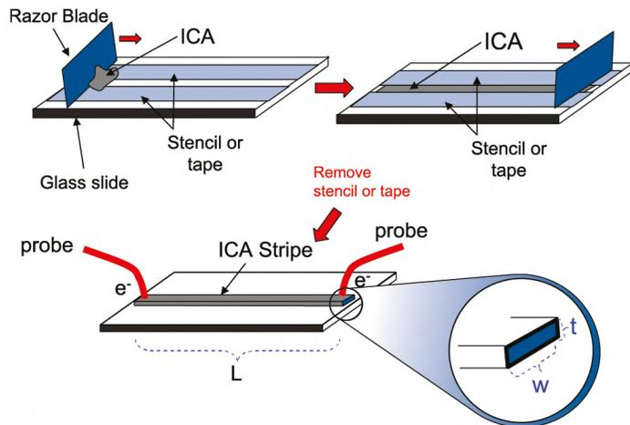
Once the sample has been prepared and cured, the two probes of a voltmeter are applied to the ends of the stripe to measure the resistance across the sample. Volume resistivity is then calculated according to the following equation:
